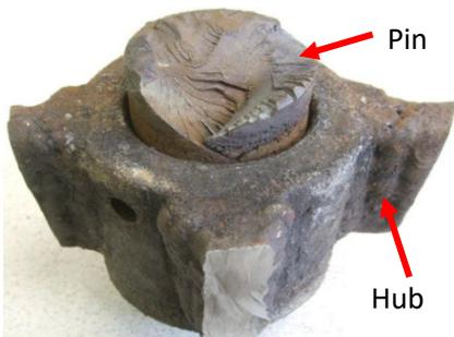
While the turntable pin may seem like a minor component, its failure can cause significant harm to all persons utilizing the accommodation ladder. In this instance, the vessel's crew was in the process of stowing the accommodation ladder when the turntable pin failed. As a result, a crewmember who was on the accommodation ladder at the time fell approximately 30 feet and sustained serious injuries.
