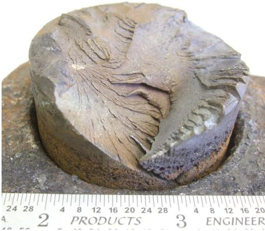
*Figure 3: Surface corrosion and contamination are evident on the fracture surface of the failed turntable pin. Severe corrosion pits and surface cracks are also visible on the sidewall, which could have provided an indicator of the pin's unsafe condition prior to failure.*
